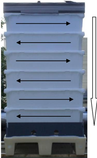
**Picture 8 Arrows illustrating direction of water flow through the unit.**
