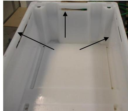
**Picture 7. Showing slits for outflow.**
