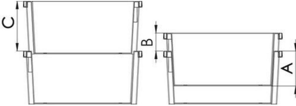
Picture 3. Box height, with and without product. 75% of total box height, A, is contained in the box below when stacked without product.
