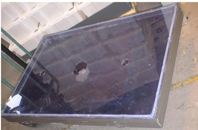
**Picture 5. Showing water inlet, and the water distribution arrangement.**
